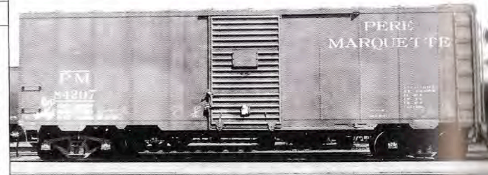
ABOVE: This in-service photo of PM No. 84207 represents the cars built by GATC from series 84200-84299. These cars received US Gypsum metal running boards and brake steps.
